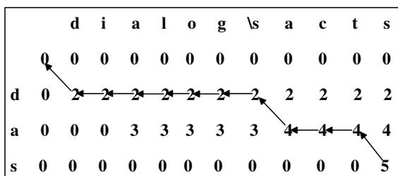
**Figure 2.** For example, the definition is “Dialog Acts”, and the abbreviation is “DAs”. All the arrows form the best match pathway.
