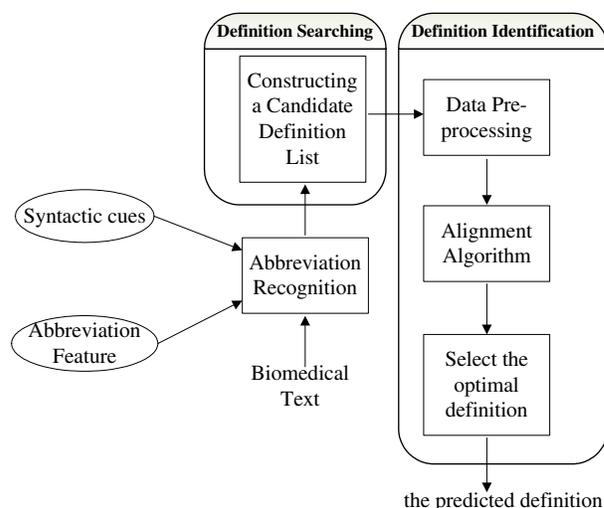
**Figure 1. This is the flowchart of extracting abbreviations and their corresponding definitions.**
